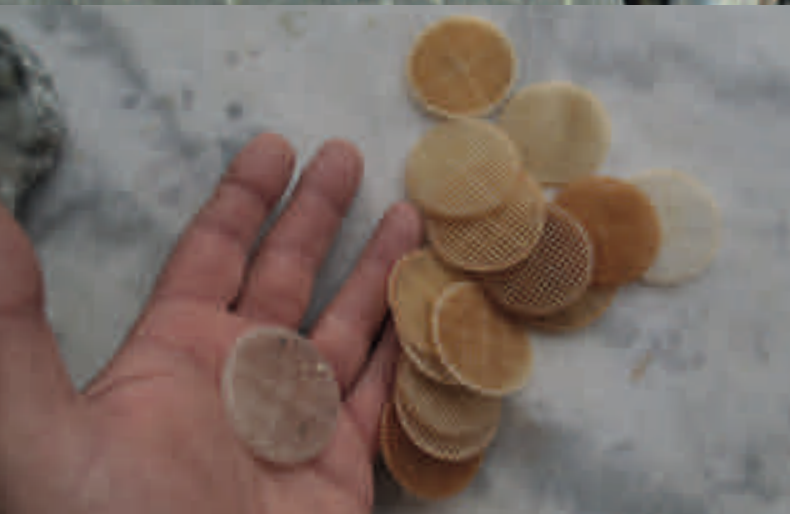
Top : K3 model biomedias washed up on the banks of the river Nive upstream from Saint-Jean-Pied-de-Port (64) Above: biomedias collected from the Var.
